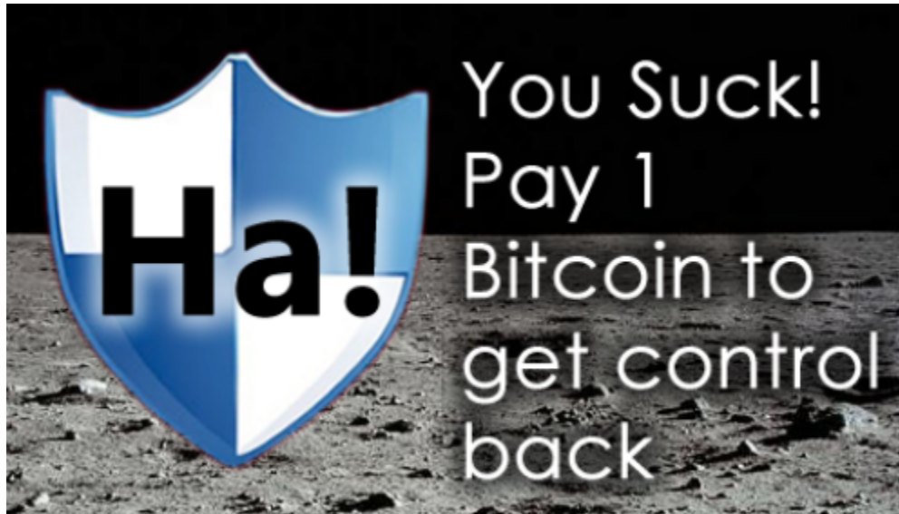
Figure 2: Ransomware message displayed on Smart-Thermostat
