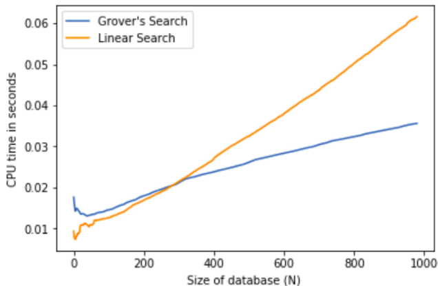
Figure 7: Average running time for Linear and Grover's Search Algorithms on HR Database
